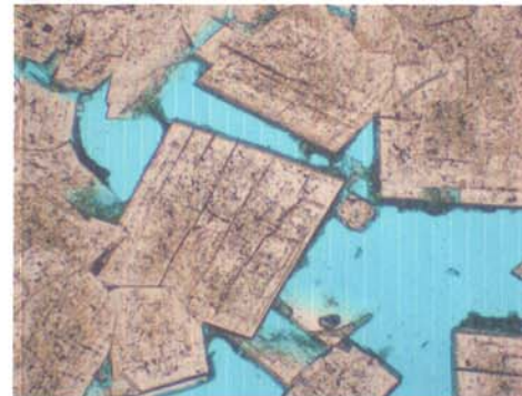
Biomould in dolomite lined by euhedral dolomite cement. 2309.95m, field of view 5mm
