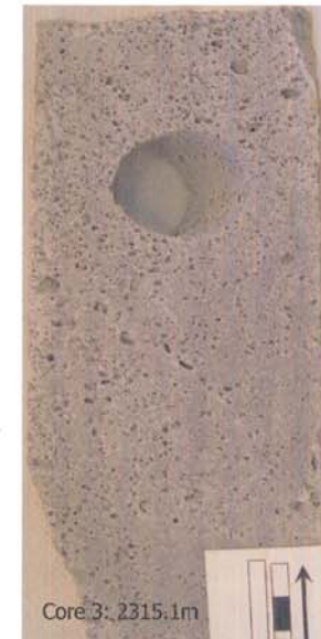
Dolograinsone with common dissolved crinoid ossicles and shell, possible cross-bedding defined by oblique alignment of biomoulds.
